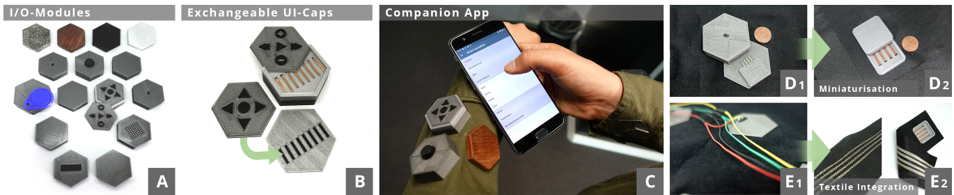
Figure 2. Our prototype comprises 15 modules (A) ranging from displays to customizable touch modules (B). This variety allows the combination of input and output modules to define custom functions with the smartphone app (C). We work on miniaturisation (D1-2) and improved integration (E1-2).
