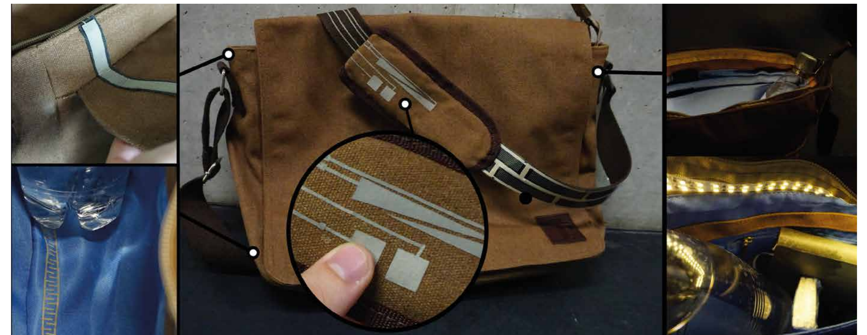
Prototype created with the RIO Toolkit: Messenger Bag with ironed-on solar cells, LEDs, capacitive controls, bend- and moisture-sensor.
