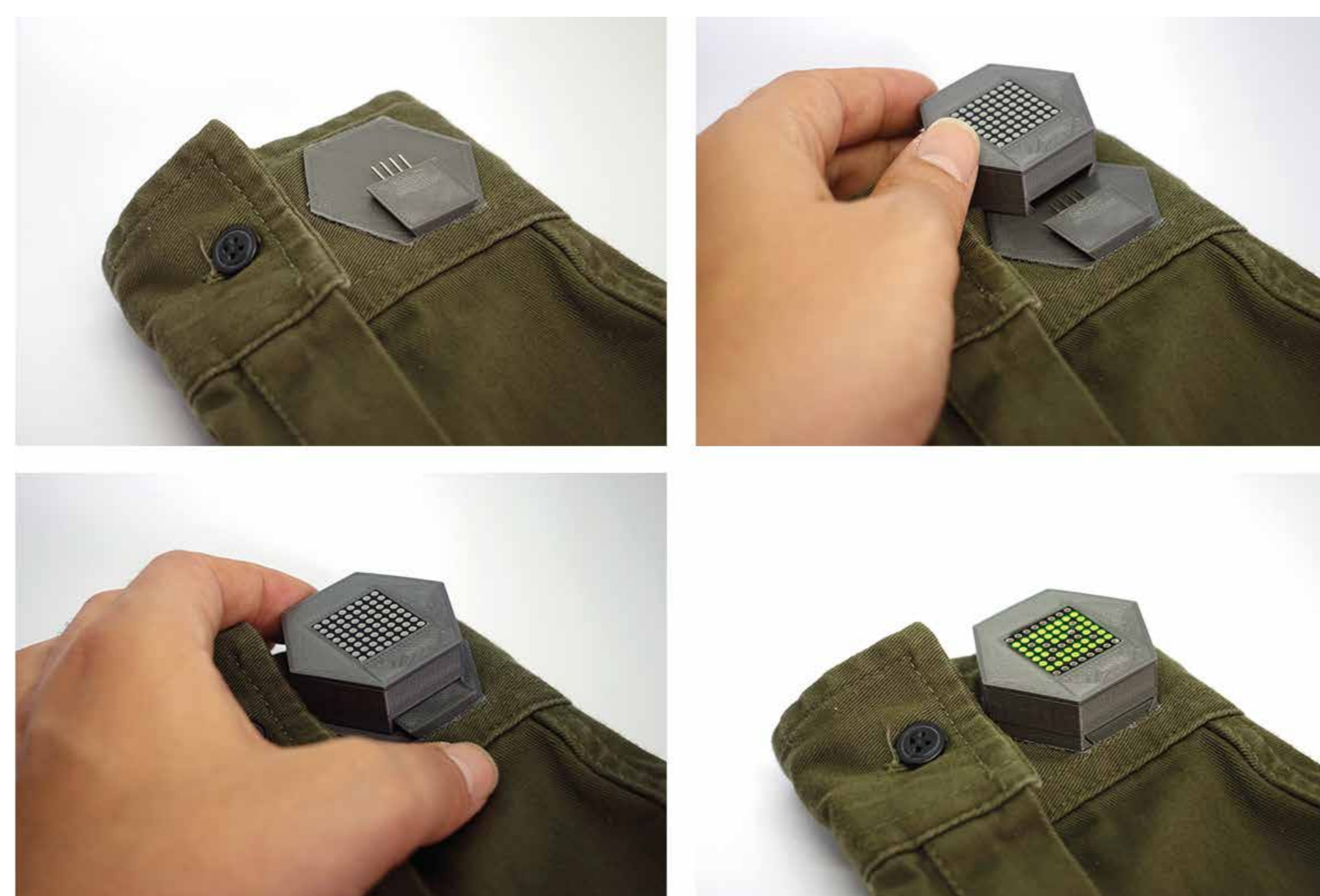
By simply clicking the modules into the embedded sockets, individual applications can be created and rearranged at runtime.
