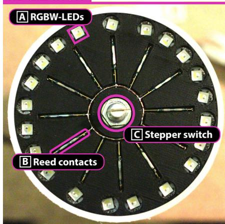
Figure 4: Important **electronic parts** of ScaleDial are RGBW-LEDs (A), reed contacts (B) and a stepper switch (C).
