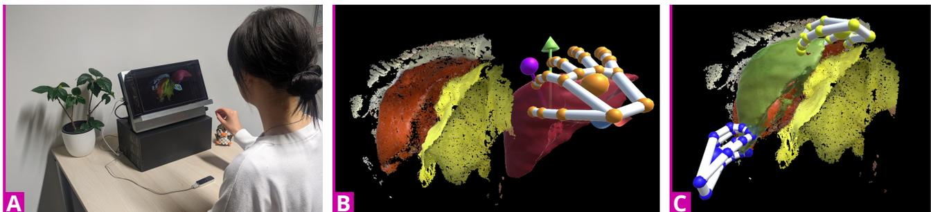
Figure 1: Our proposed and implemented system for the manual point cloud alignment. (A) shows a user interacting with the system consisting of a stereoscopic display and hand tracking device. (B) displays a point cloud (left) and a solid model (right). The model can be interacted with directly or via attached handlers. In (C) the same model is scaled by the use of both hands.
