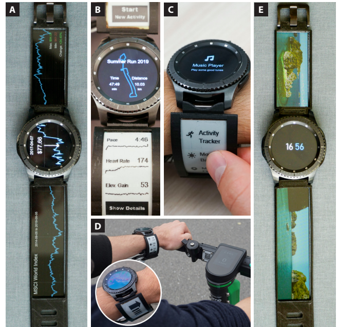
Figure 1. StrapDisplays allow for extending commodity smartwatches into a Watch+Strap system; this enables, e.g., expanding information spaces (a+b), easy-to-reach quick access menus (c), glanceable information while on the go (d), or displaying high-resolution content (e).
