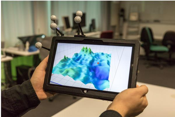
**Figure 1:** One of our prototypes, showing a 3D height map fixed in space and explored by spatial interaction.
