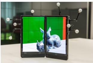
**Figure 4:** Two connected devices with a scene fixed in space and head-coupled perspective. The picture is taken from the tracked user's point of view.
