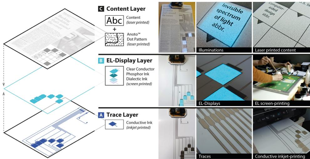
Figure 2: **Fabrication process:** Our completely printed IllumiPaper sheets consist of three layers: A conductive printed trace layer (A), a screen-printed EL-display layer (B) and a digital pen-enabled content layer (C).
