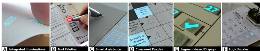
Figure 1: IllumiPaper integrates visual feedback for digital pens on standard paper by using novel thin-film technologies. We demonstrate a research platform with completely printed, paper-integrated illuminations.
