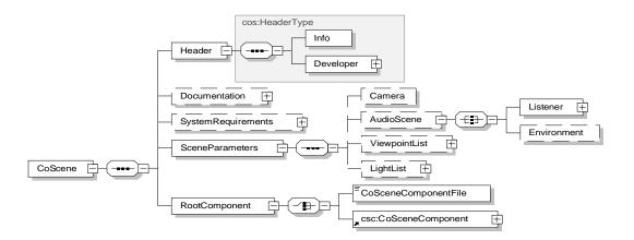
Figure 6. Structure of XML schema CoScene
