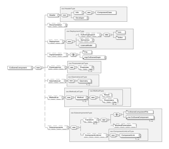
Figure 5. Structure of XML schema CoSceneComponent
