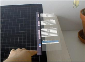
**Figure 3:** *DesignAR*: Menu offloaded in AR space with the display's borders used for interaction.
