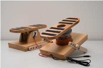
Figure 4: Foot-joystick & Foot-rocker setup
