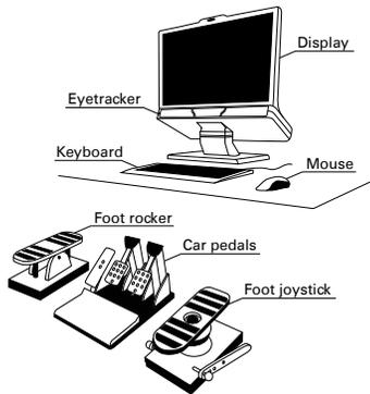
**Figure 1:** Extended desktop workplace with our proposed input devices.
